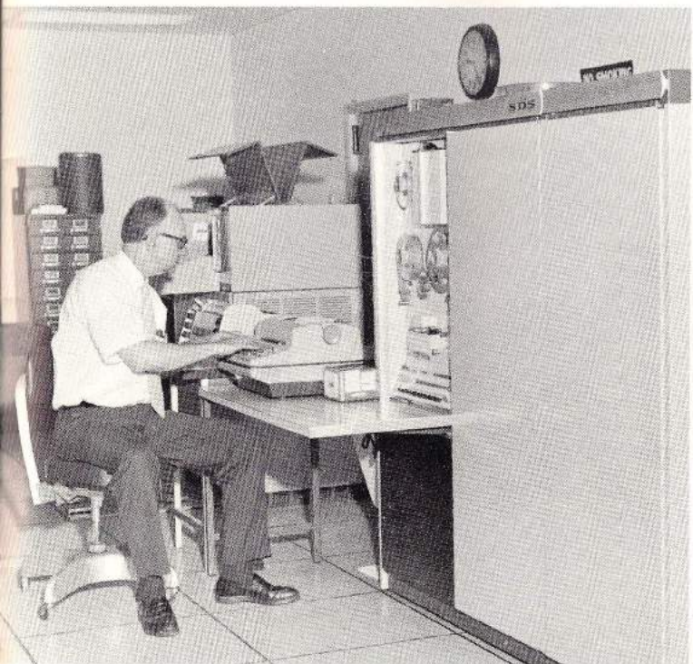
SDS 920 Computer Console & Central Processing Unit.
