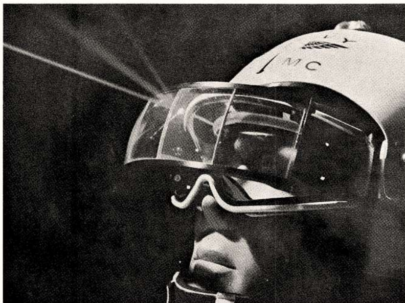
Demonstration picture of how visor reflects laser.
